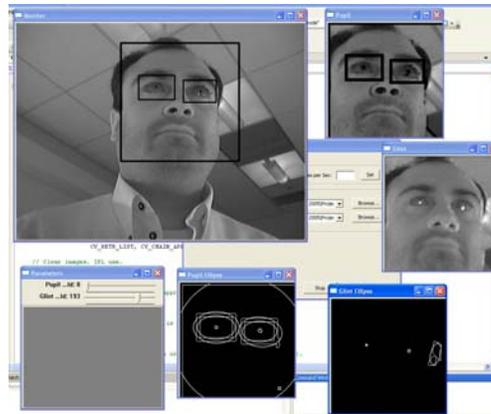
GazeTracker software built on open source Computer Vision libraries (OpenCV) uses machine learning to identify faces in the image and then looks within the face region to identify eyes. Simple image processing (erosion/dilation) help to separate the pupil and the glint images. Ellipse-fitting provides the center of the pupil and the glint. The relative position and distance of the glint will then be used to determine the gaze vector.
