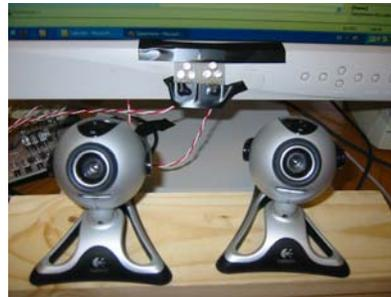
Prototype in development uses commercial-over-the-shelf cameras modified to work in the infrared spectrum and low-cost parts such as IR LEDs.
